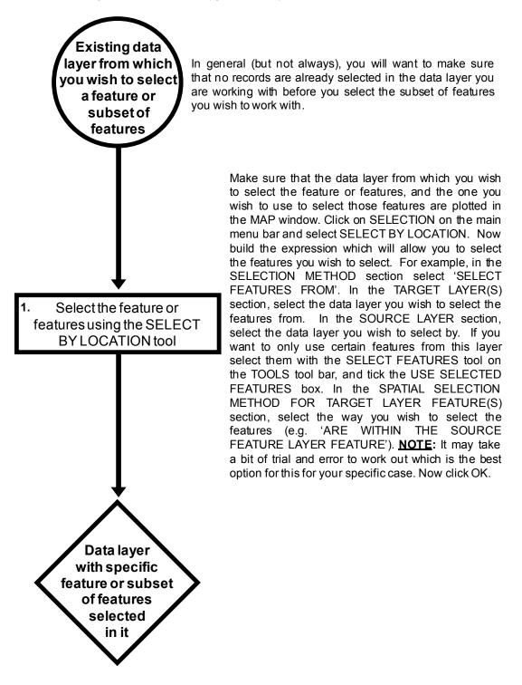
To select a subset of features in a data layer using the contents of its attribute table, work through the following flow diagram:
