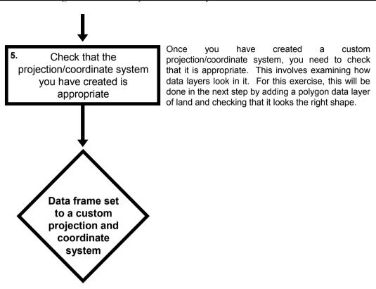
To check that you have done this step properly, right click on the name of your data frame (LAYERS) in the TABLE OF CONTENTS window and select PROPERTIES. Click on the COORDINATE SYSTEM tab of the DATA FRAME PROPERTIES window and make sure that contents of the CURRENT COORDINATE SYSTEM section of the window has the following text at the top of it:
